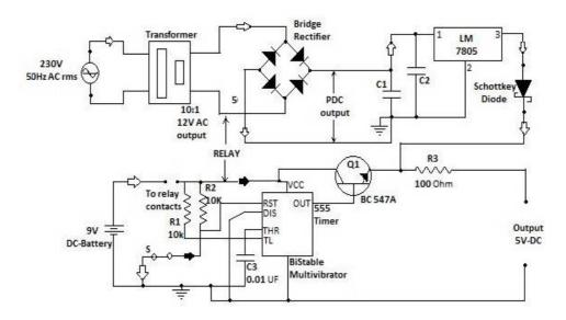
Fig. 2 Automatic Change over Circuit.
